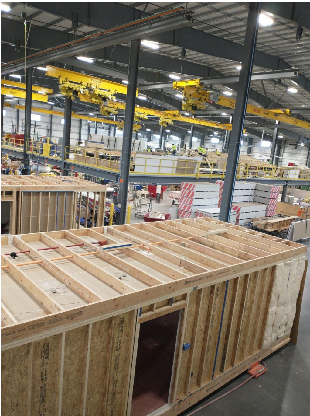
Fading West started building "off-site" homes for its own project, The Farm, in Buena Vista. Scott Miller/smiller@vaildaily.com
